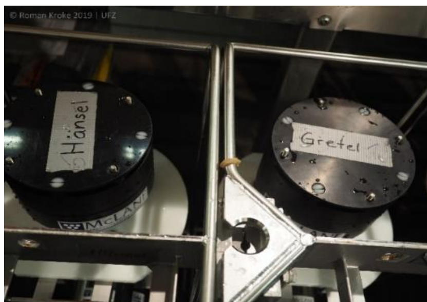
The in situ pumps Hansel and Gretel.
