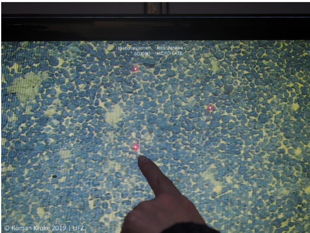
A seabed littered with manganese nodules. The three red laser dots allow a correct classification of the size ratios.
