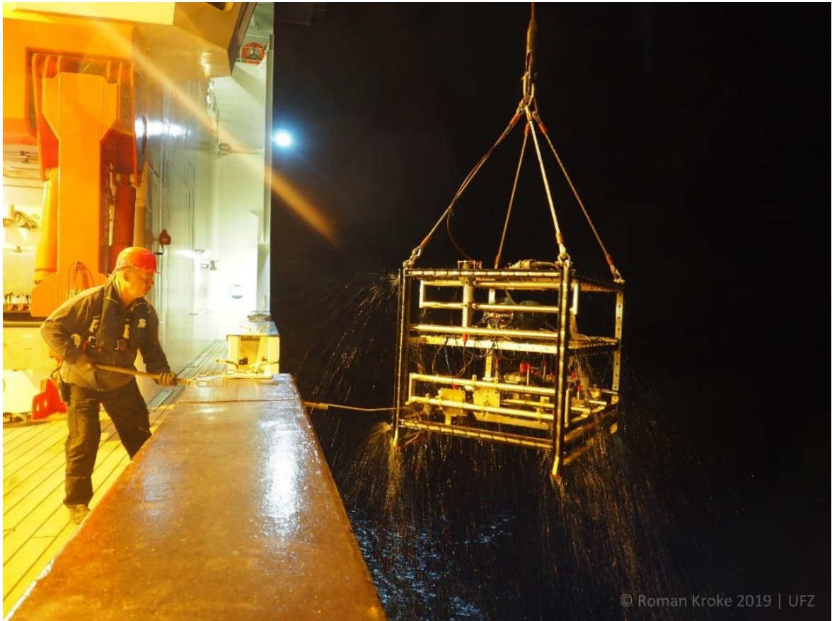
Our "deep-sea eye" OFOS comes back from the seabed with photos from more than 5000 metres depth..
