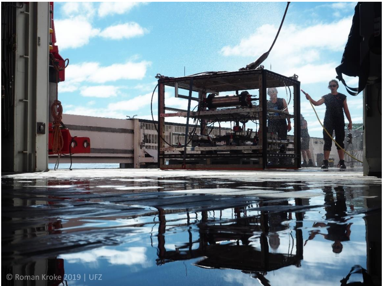
The remote-controlled camera system OFOS (Ocean Floor Observation System).
